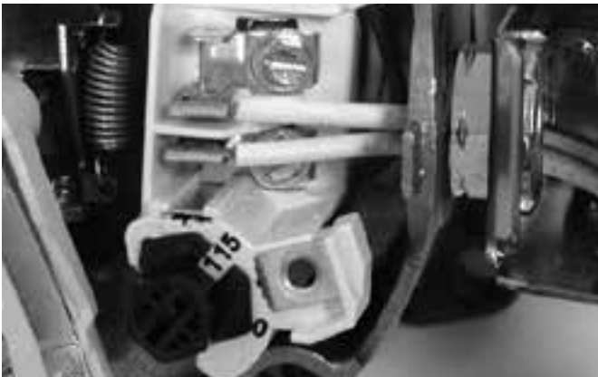
Figure 7: Voltage set to 115 volts, Dial Type
